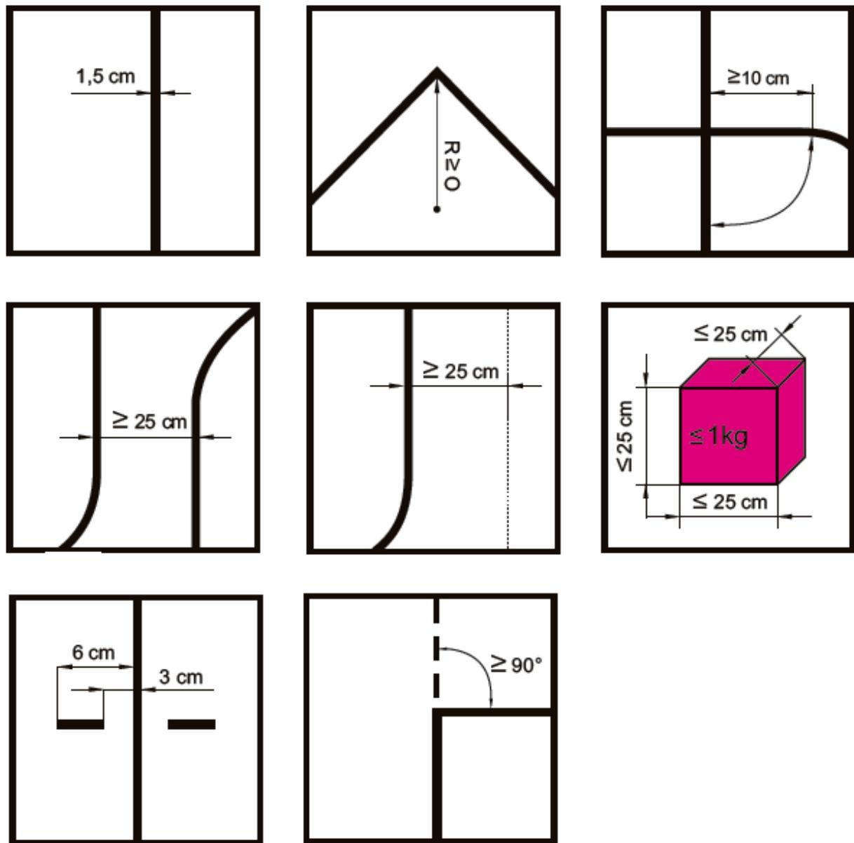
Figure 1: The dimensions of the track and robot.
